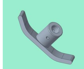
FIGURE 98: SLED FOOT DESIGN
