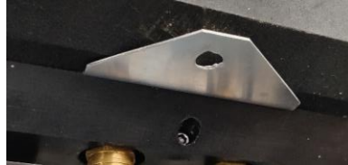
FIGURE 12: TETHER CONNECTION LOOP
