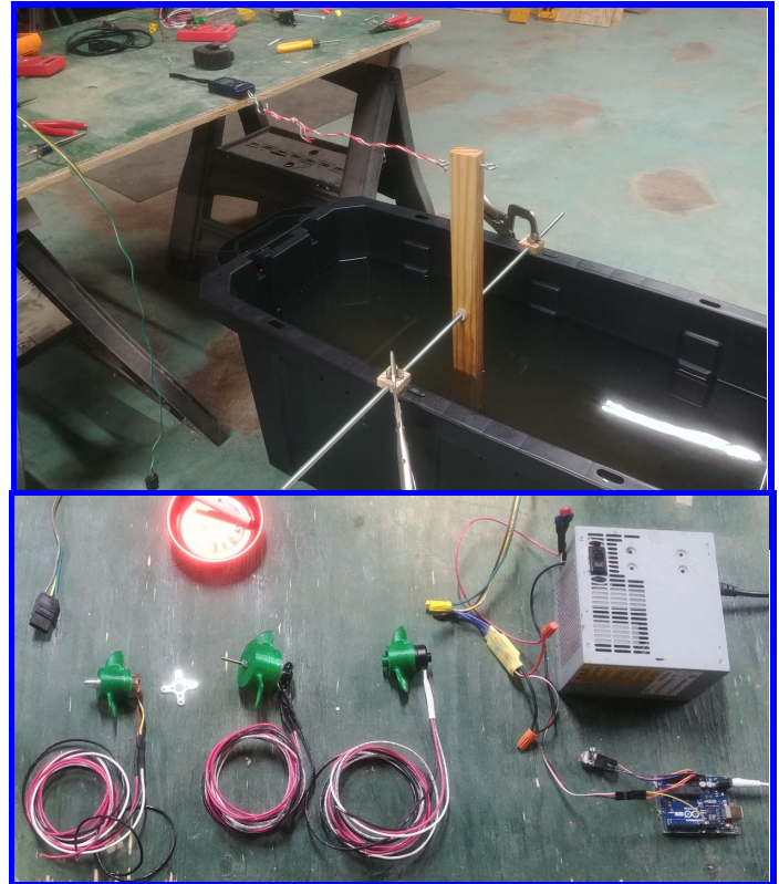
Figure 2.1 Thrust/current testing setup
