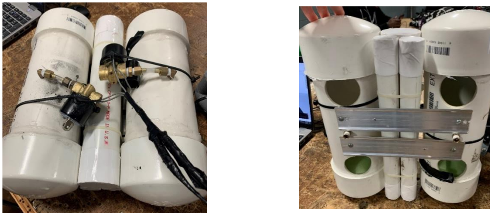
Figure 11 – Maximus' Ballast Tanks
