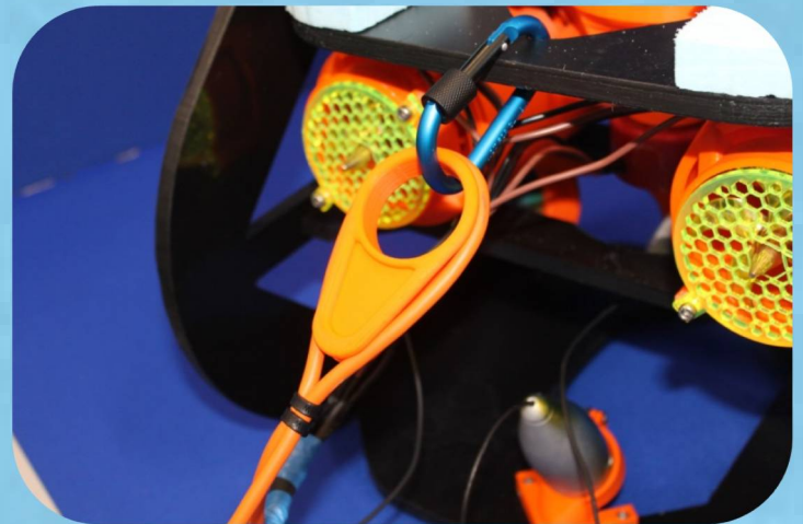
The strain relief on Aegaeon which keeps our tether safe - Dylan Taylor
