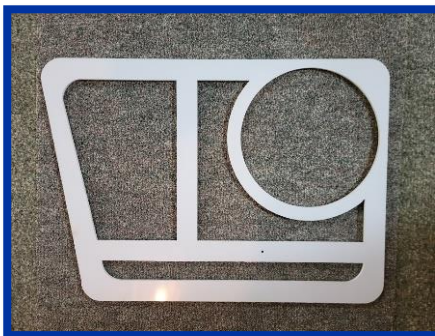
Figures 16, 17, 18 left to right: Side frame piece cut from PVC. Scale frame prototype. 3D printed bottom base plate. Photo Credit: Melissa Lewis
