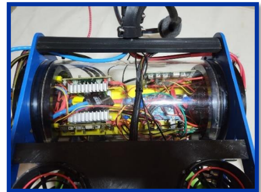
Figure 5: Onboard Electronics using a Blue Robotics Tube Photo Credit: Melissa Lewis
