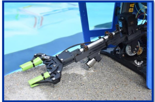
Figure 22: Custom designed manipulator. Photo Credit: Melissa Lewis
