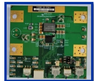
Figure 6: Vicor 48V to 12V switching regulator. Photo Credit: Melissa Lewis
