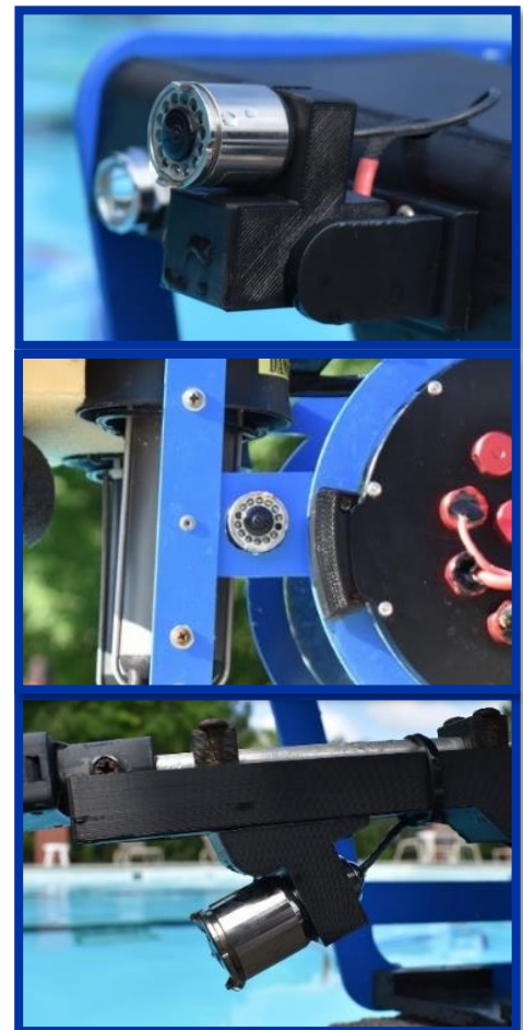
Figures 23,24,25 Cameras Top: Front main camera on custom tilting mount. Middle: Side View camera Bottom: Camera installed on manipulator Photo Credit: Melissa Lewis
