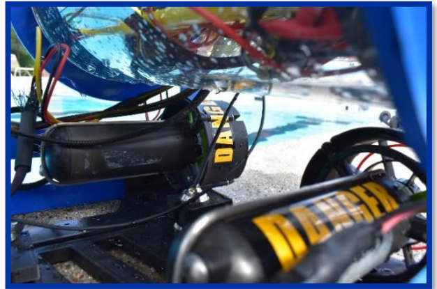
Figure 20: Forward/back thrusters mounted on ROV baseplate. Photo Credit: Melissa Lewis
