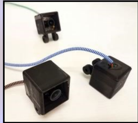
Figure 2.3.1: The cameras in 3D-printed housings.
