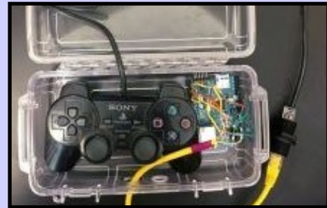
Figure 2.6.1: ROV Controller and sender Arduino.
