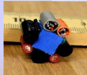
Figure 2.2.1: Cross-section of tether.
