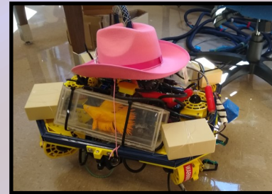
Figure 2.8.1: One of two buoyancy boxes.
