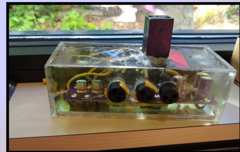
Figure 2.9.1: Power conversion board.
