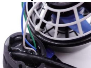
Figure 11 Thruster ESC casted in housing
