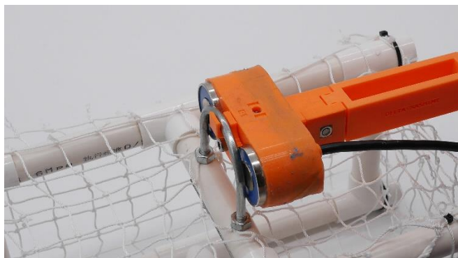
Figure 24 Bi-EM and U-bolt hook holding eel trap
