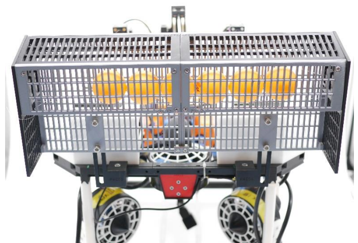
Figure 31 Surface Debris Collector
