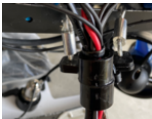
Figure 29: Safety measures implemented on ROV include no sharp edges, danger labels on thrusters, tether restraint and epoxying wires for watertight seal.
