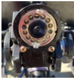
Figure 24: Main camera mounted on tilt mechanism
