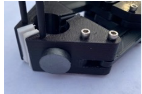
Figure 19: Magnet attached to gripper for pin removal
