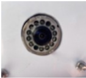
Figure 23: Baseplate camera for viewing transect line
