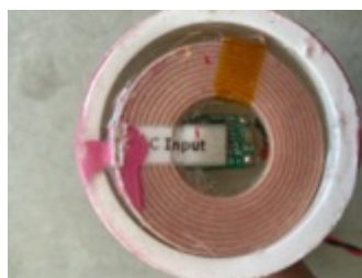
Figure 21: Pictures of Seabin power connector, transmitter side of inductive coupling power and tether wire to surface power supply
