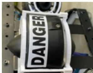
Figure 29: Safety measures implemented on ROV include no sharp edges, danger labels on thrusters, tether restraint and epoxying wires for watertight seal.
