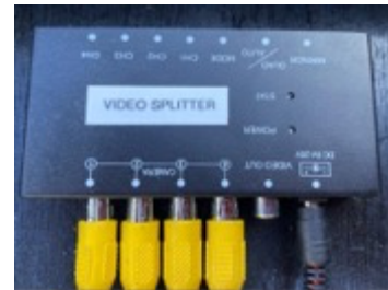
Figure 25: Video splitter, allowing multiple cameras to be viewed on one monitor
