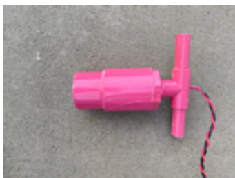
Figure 21: Pictures of Seabin power connector, transmitter side of inductive coupling power and tether wire to surface power supply
