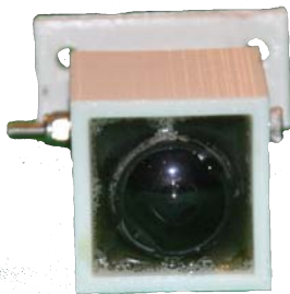
Figure 10: Drone camera, waterproofed in 3D printed box
