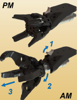
Fig. 12 - The quick-detachable Primary and Auxiliary Manipulators
