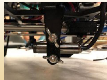
Fig. 9 - An USB camera in its adjustable mount
