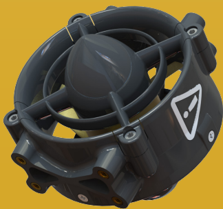
Fig. 4 - A horizontal thruster, featuring custom-printed ducts with integrated safety shrouds and warning placard
