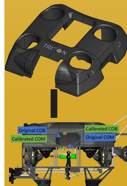
Fig. 11 - The initial COM and COB, along with the tuned COB and COM
