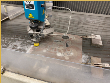
Fig. 3 - Water-Jetting a frame plate
