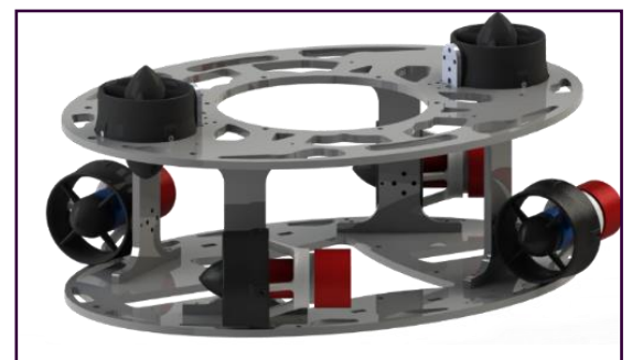
Figure 10. Oogway's Thrusters' Configuration
