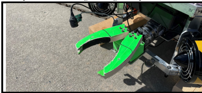
Figure 6: Stand-alone manipulator on “Hammerhead.” This system is featured on both the front and rear of the system.
