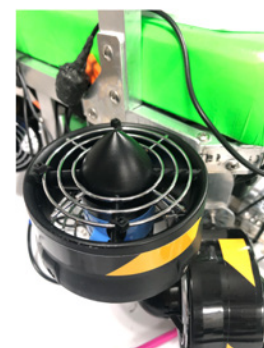
Figure 22: Safety shrouds installed on all thrusters.
