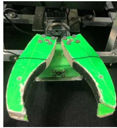
Figure 16: Gripper jaws with grip tape glued in place. Green worm gear box and planetary gearbox is visible as well.
