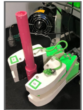
Gripper claw adapters used for coral transplanting.
