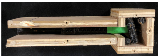
Figure 11: “Gripper Analog” built to match size and weight of gripper, to allow buoyancy testing even while the actual grippers were still under construction.
