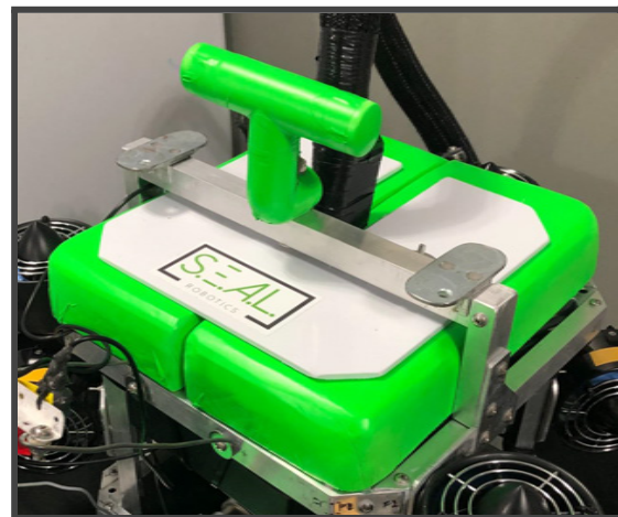
Figure 2: ROV Handle Pictured.
