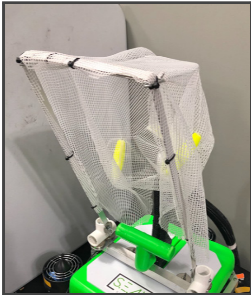
Magnetically mounted surface plastic collection device. Easy debris collection and removal. Other tooling devices use the same magnetic mounts on the ROV.
