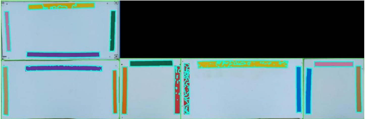
Photomosaic output with hue based tape identification (All images by Jenna Li)
