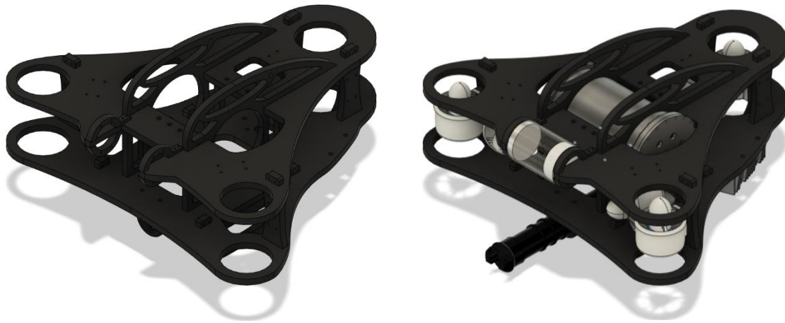
Fig. 2 – 3D model of chassis and full ROV composition in CAD program.
