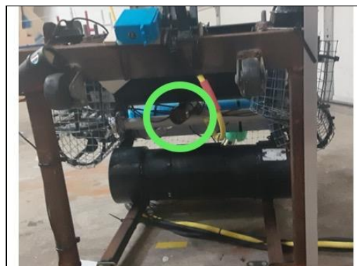
Figure 18: Downward facing camera (camera #5, green circle) provides view of appropriate regions when flying transect.
