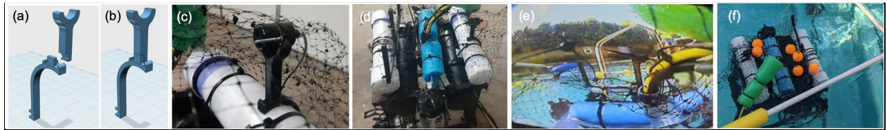
Figure 17: Custom mounted camera for improved surface viewing. A custom 3D printed camera mount was made to mount the camera above the ROV. This camera is essential to collecting debris from the water’s surface. With this mount, if the ROV is positioned as the surface for surface trash collection, the camera is above the water, providing a clear view of surface debris and avoiding a situation where the camera dips in and out of the water leading to poor optics. (a,b): design for camera mount, (c,d): mounted camera, (e): view from camera, (f) successful camera-guided collection of surface debris.
