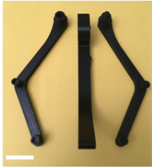
Figure 11: Third Generation Claw. The white scale bar shown in the lower left represents a length of 2cm. This claw was able to perform most tasks and was used for the World Championships Qualifier. However, the connectors were flimsy and it quickly broke and was replaced with a sturdier design (fourth generation claw).
