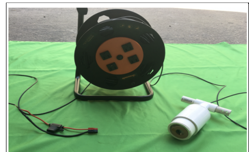
Figure 8: Tether management device used to minimize the risk of the non-ROV power cord tangling with itself or the ROV tether
