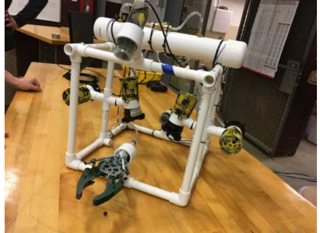
Image 1.5: The ROV and the motors
