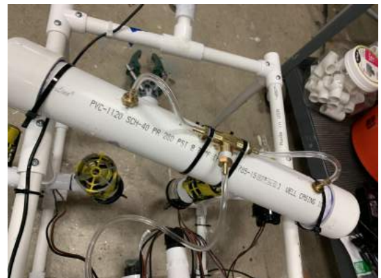
Image 1.6: Variable Ballast Tank
