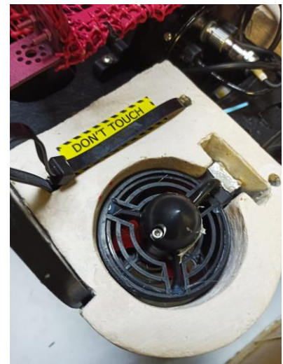
Fig. 19 IP20 thruster propeller protection
