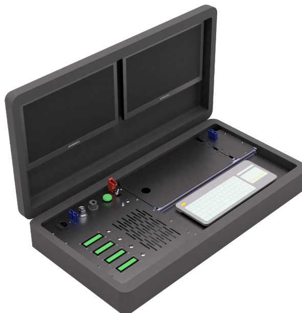
Figure 8: Surface control station CAD render.
