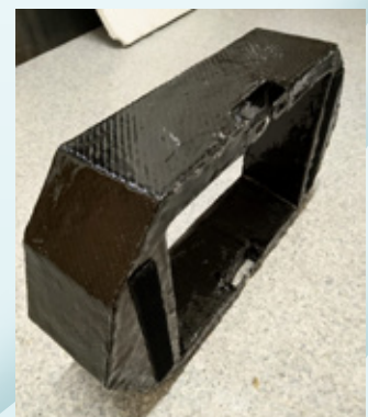
Figure 8. Buoyancy embedded with L-shaped connector and Dual Lock
