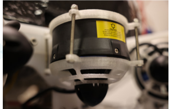
Figure 41. Shrouded thrusters with warning labels
