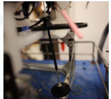
Figure 35. Lock with a bended elastic rod
