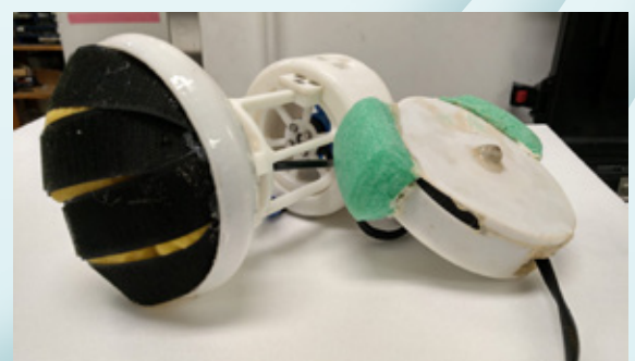
Figure 33. Micro-ROV with cable reel
