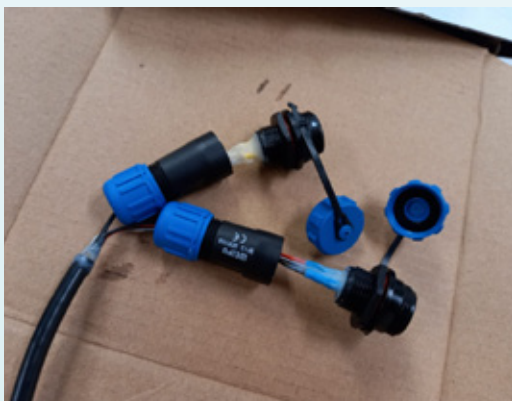
Figure 15. Epoxy between wires and headers
