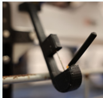
Figure 36. V-shaped hook picker
