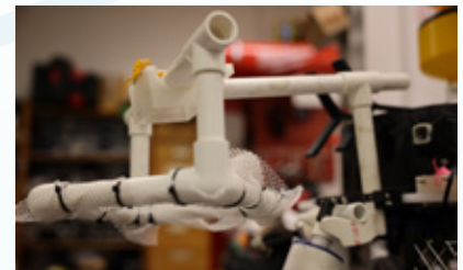
Figure 20. Releaser with mesh bag and power port
