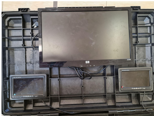
3 monitors mounted onto the lid of the control box
