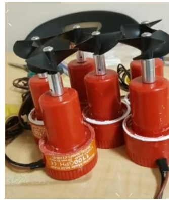
Modified bilge pumps with propellers
