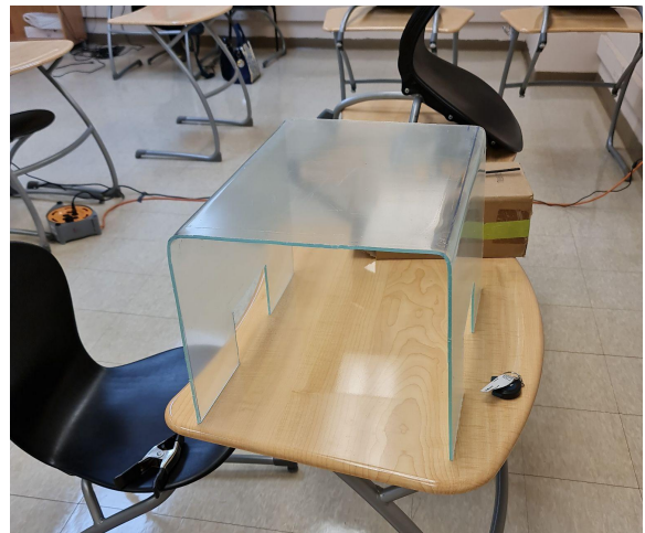
ROV chassis designed from a single sheet of bent acrylic
