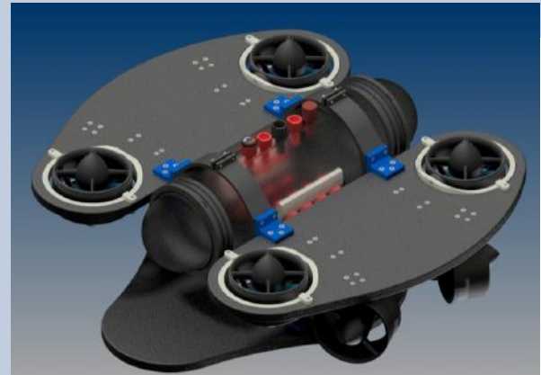
Figure 4: Original CAD of the SousaSub frame
