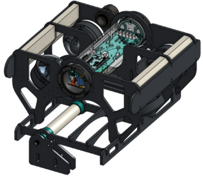
Fig 3: The ROV ANT CAD design.
