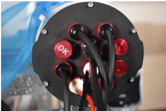
Cables entering tube and wire rope connected to eye bolt for strain relief. (Photo Credit: Nathan Madsen)
