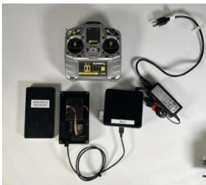
Top-side electronics with RC transmitter and receiver, Arduino and Intel NUC. (Photo Credit: Nathan Madsen)
