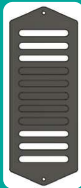
Figure 8 (left): Foam mounting platform modeled in Fusion 360.
