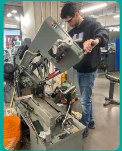
Figure 4 (top) and 5 (bottom): Bandsaw and mill at Brunsfeld Center being used to prepare the frame's aluminum channels.
