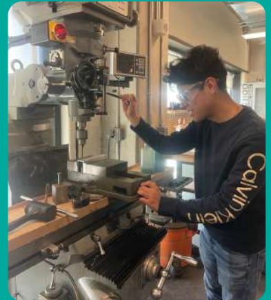
Figure 4 (top) and 5 (bottom): Bandsaw and mill at Brunsfeld Center being used to prepare the frame's aluminum channels.
