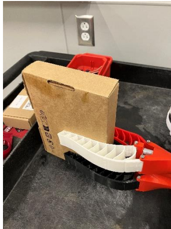
The gripper grabbing a large box in the vertical direction
