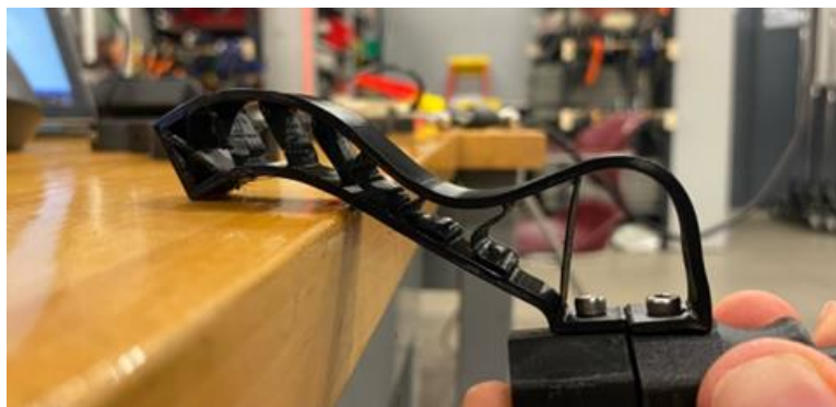
A finger deforming around a solid object
