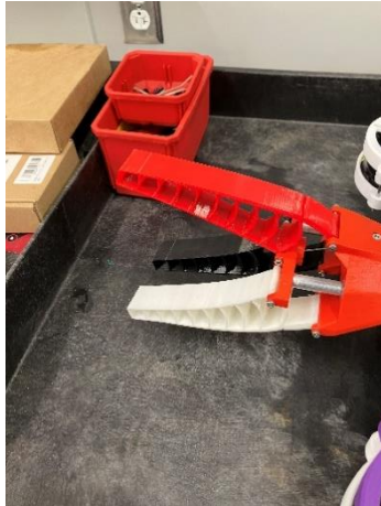
The gripper in the open position
