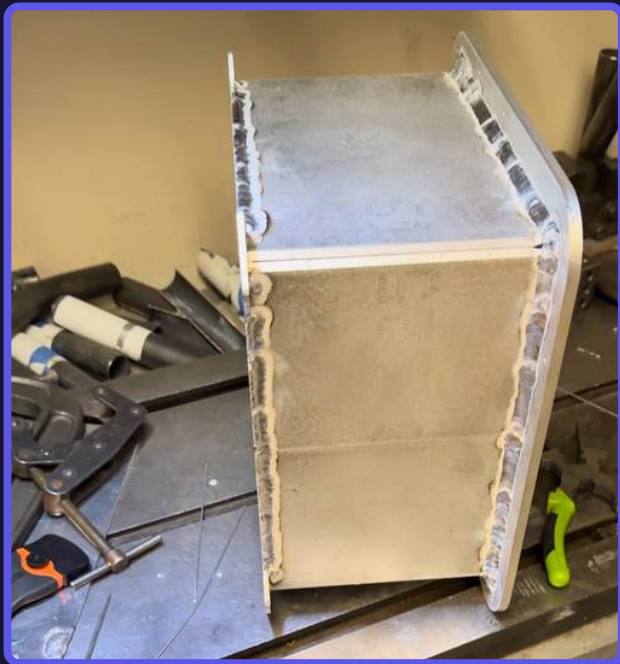
Figure 29: Partially Welded Ebox
