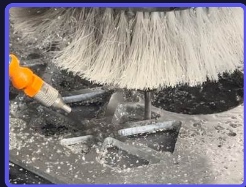
Figure 25: CNC Router Cutting Pocket Plate
