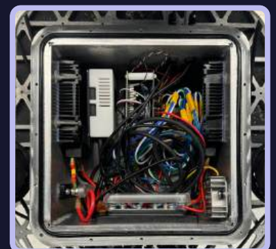
Figure 11: Wire Routing Inside EBox
