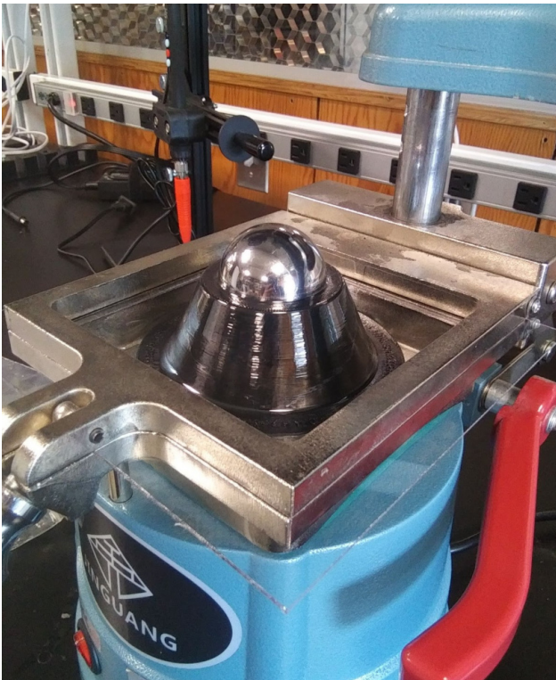
Figure 15: In-house dome vacuum forming process (left), Flir camera with enclosure (top right), rotating Luxonis stereo camera (bottom right)
