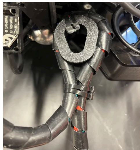
Figure 31: Tether support where the tether connects to the ROV
