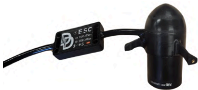
Figure 5: Spare Thruster Core Used for Claw Motor
