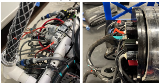
Figure 6: Our old wire management entering the tube (Left) vs our new wire management (Right)
