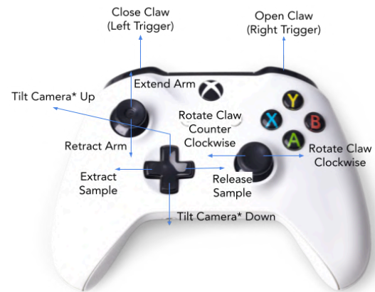
Figure 25: ROV Control Scheme: Claw Controller
