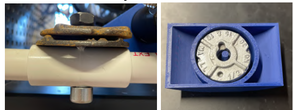
Figure 15: Old and new modular ballast system
