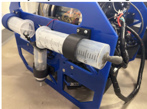
Figure 14: Adjustable syringes for buoyancy By filling the syringes with air and capping them before submersion, the syringes act as adjustable buoyancy tanks that can be
