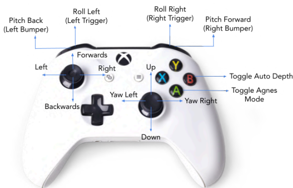
Figure 24: ROV Control Scheme: Main Controller
