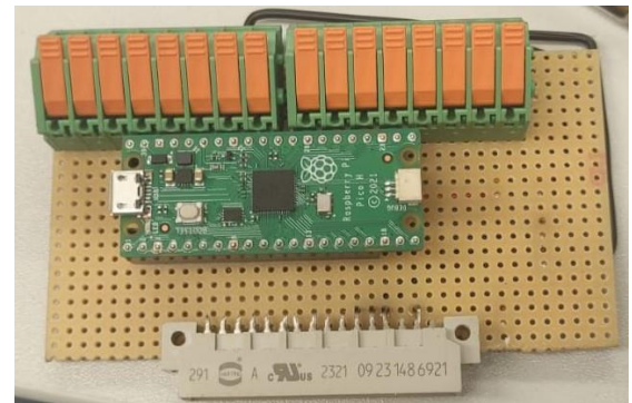
Figure 9: Improved Hotswap Module based on the Pi Pico.
