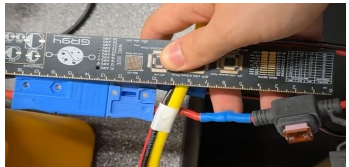
Figure 15: 30A fuse placed roughly 10cm away.
