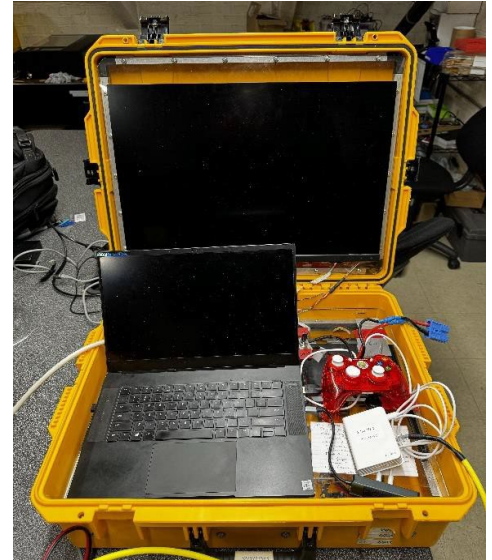
Figure 13: Surface Station for joystick controls
