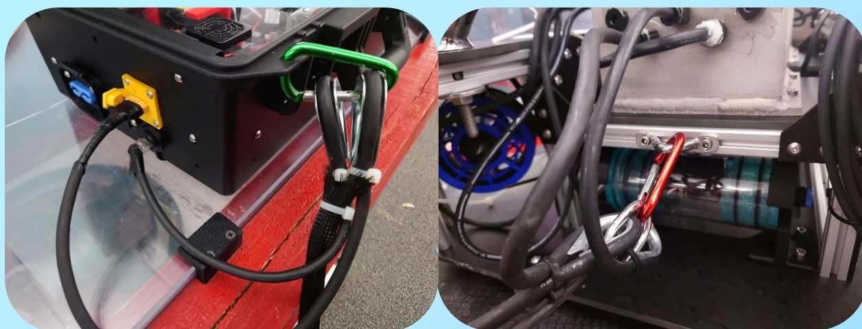
Figure 3. Strain Relief. Left) Topside Strain Relief. Right) ROV Strain Relief
