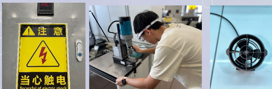
Figure 20 (left) Warning Label, (mid) Safety glasses, (right) Thrusters guards
