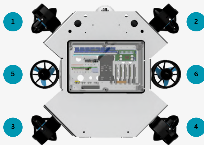
FIG 8 : T200 Thruster Placement and ROV Movement/DOF.
