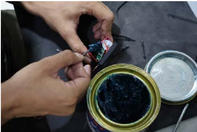
Figure 35. Waterproofing servos process
