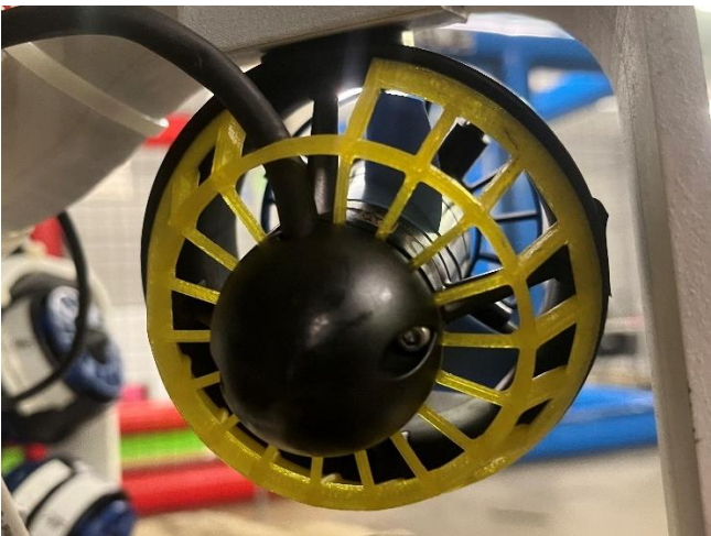
Figure 9: Image showing thruster equipped with propeller guards. Credit: Matthew Smith.
