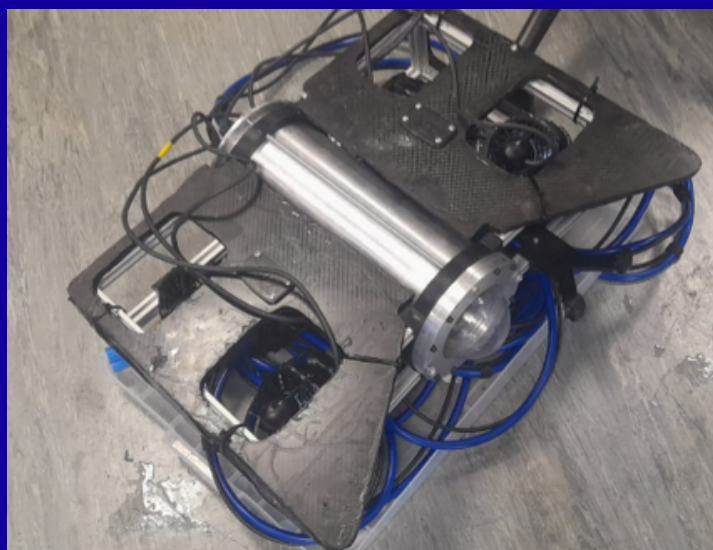
Figure 2: Photo of ROV excluding buoyancy tubes & dynamic actuation tools.
