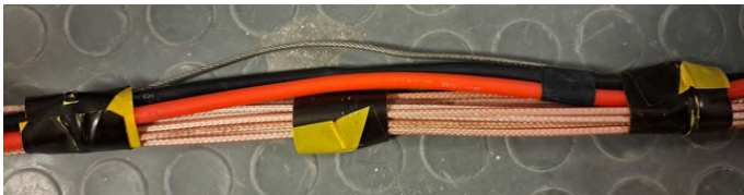
Figure 15. SDI cables, AWG cables, and strain relief
