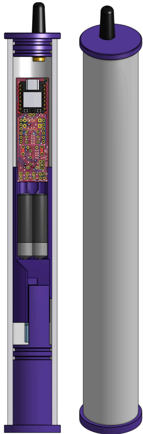
Fig. 17. Nanofloat 1.1 Section View (Left) and Isometric View (Right)
