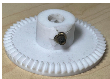
Fig. 20: Failure mode discovered through testing.
