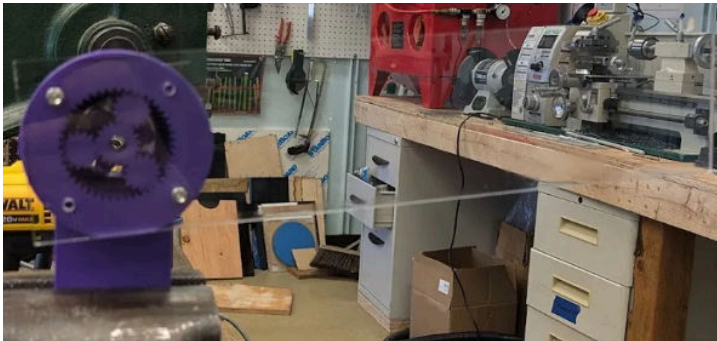
Fig. 19: Gearbox testing setup.
