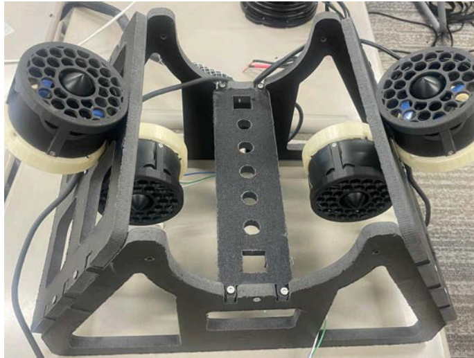
Figure 4: Cuesta AquaCats HDPE Assembled Frame (cut by waterjet)
