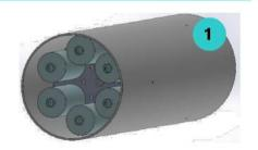
This autonomous device has been designed to operate in aquatic environments without being connected to an ROV, with the goal of collecting key environmental data such as pressure and voltage for later analysis. Its modular design clearly separates the electrical systems, sensors, batteries, and mechanical components, optimizing both maintenance and safety during operation. The cylindrical housing, made of 3D-printed PVC, is optimized for vertical movement and is corrosion-resistant.
