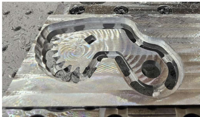
Aluminum Gripper Linkage During Machining Process
