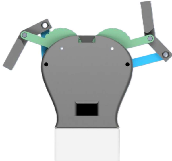
Render of Gripper Mk 1 in Crossed-Linkage State
