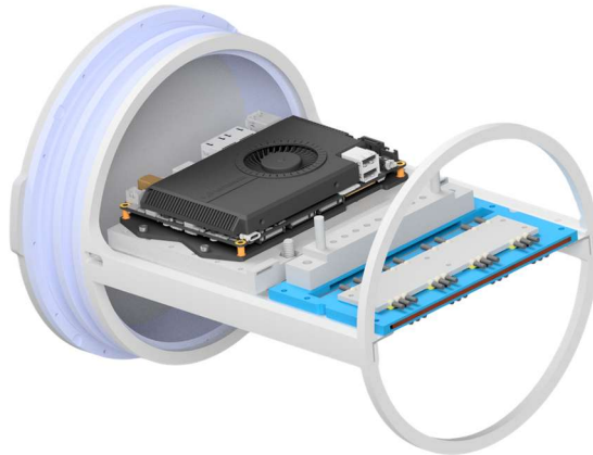
New Electronics Tray Design
