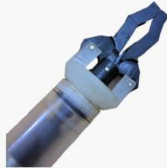
Fig. 9: Pincer , Scorpion's secondary gripper
