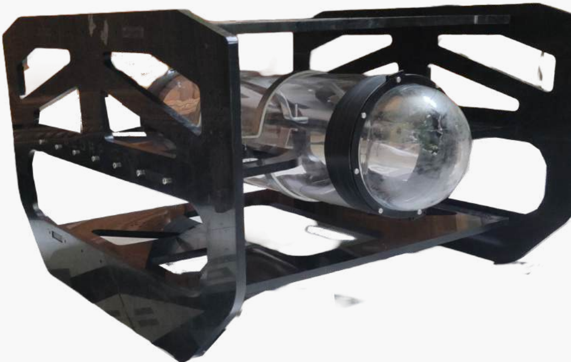
Fig. 4: HyDRA Scorpion Initial Chassis Frame Fully Assembled
