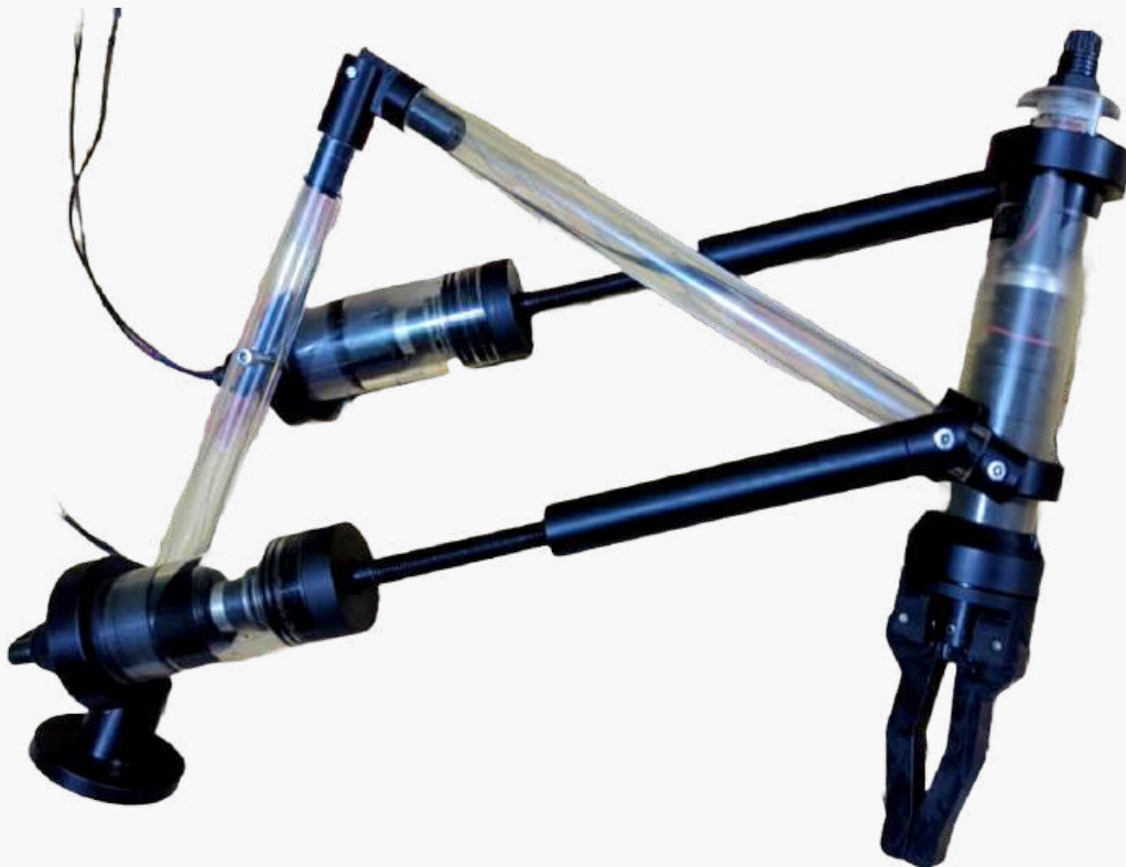
Fig. 8: Stinger , Scorpion's main manipulator arm
