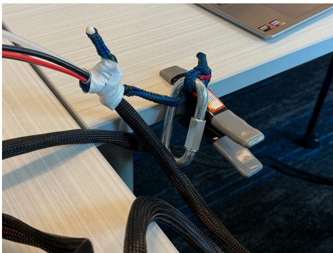
Fig. 4: Strain Relief for Top Side
