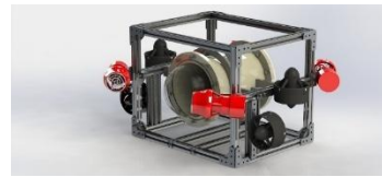
Figure 5 Full ROV frame structure designed by Mohaned Rafea using SolidWorks
