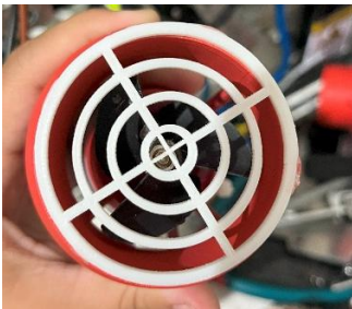
Figure 30 Bilge pump 3D printed mesh to ensure safety shot by Sarah Ateya
