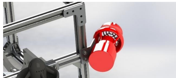
Figure 9 bilge pump fixation to Cronus's frame structure designed by Mohaned Rafea using SolidWorks.
