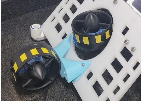
Figure 14: The mounted thrusters By Gavin Quijano
