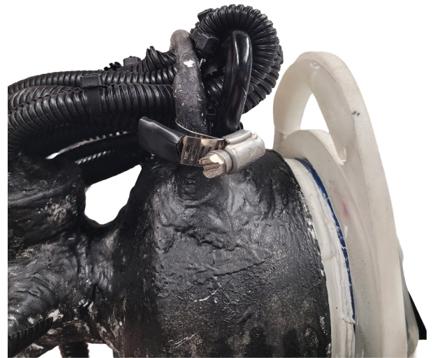
Figure 7: Completed tether strain relief system By Gavin Quijano
