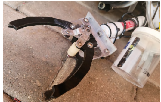
Figure 16: The claw grasping mechanism By Gavin Quijano
