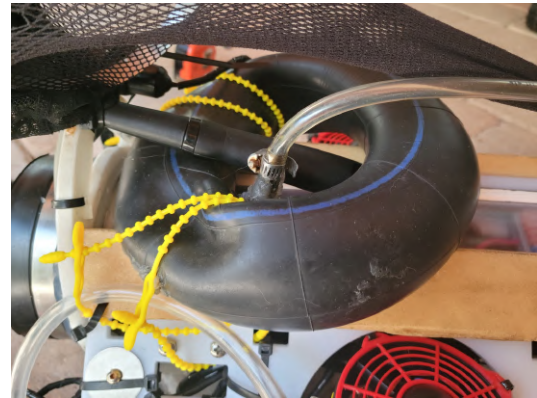
Figure 17: The variable buoyancy system By Gavin Quijano
