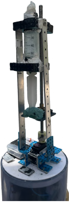
Figure 19: The buoyancy engine By Bryce Phuphanich
