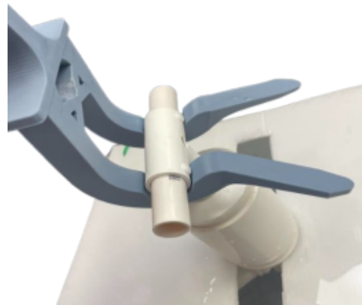
Figure.3.5.6 Photo of The second "anode hook" completing the "sacrificial anode" mission
