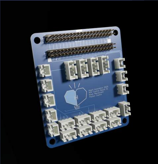
Figure 19. 3D Render of CAPTAIN’s Custom PCB
