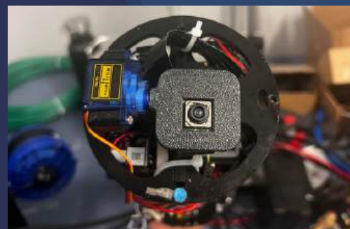
Figure 25. CAPTAIN's Front Camera.
