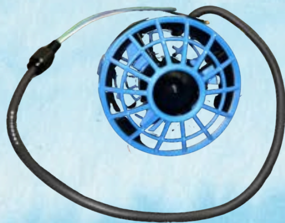
Figure 17: T200 Thruster with 3D printed Shrouds- Photo taken by Audree Alvarado
