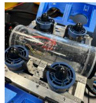
Vertical Thrusters viewed with ROV panels open for easy access. Photo Credit: Emma Schroeder
