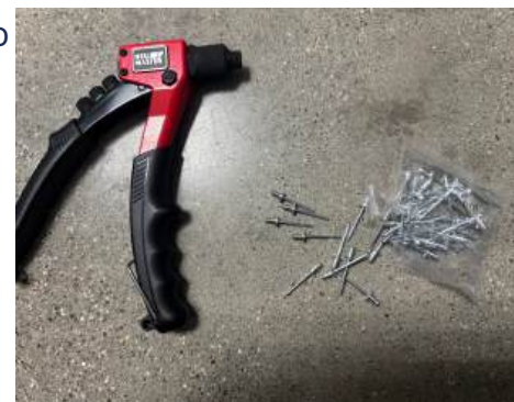
The rivet gun and rivets, we used to put our robot together.
