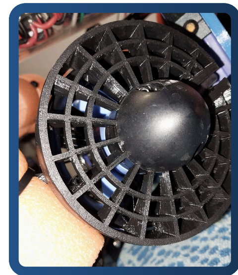
Fig. 3.6 - T200 Thruster Mounted to ROV, Jaron Cobble
