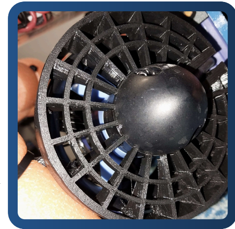
Fig. 4.1 - T200 Thruster with Shroud, Jaron Cobble
